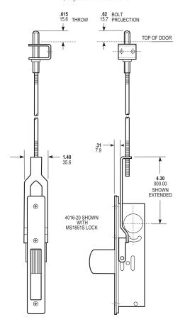
INSTALL ADAPTOR ARM TO LOCK FROM TOP WITH BOLT RETRACTED AS SHOWN, INSTALL PIN THROUGH SLOTS IN LOCK SIDE PLATES, PASSING THROUGH HOLES IN BOTH SIDES OF THE ADAPTOR ARM.
