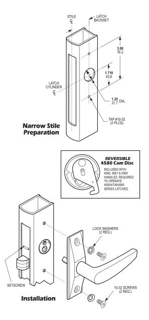
Pre-handing can be specified LH or RH although re-handing in the field is easily accomplished. The three standard handles shown are for 1-3/4" thick doors. Available on special order for doors up to 3-1/4" at extra cost.
